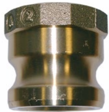
Type A Camlock x BSPP Female
