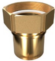
Brass DIN2817 Female BSP c/w Smooth Tail
